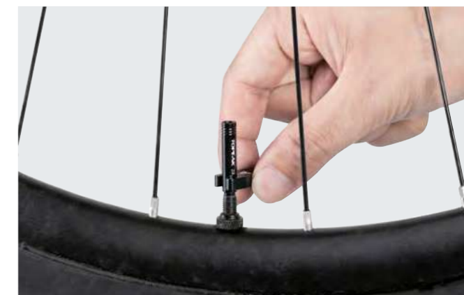
Use Valve Tool to tighten valve extender
