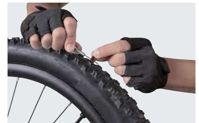
2. Remove excess plug with knife
