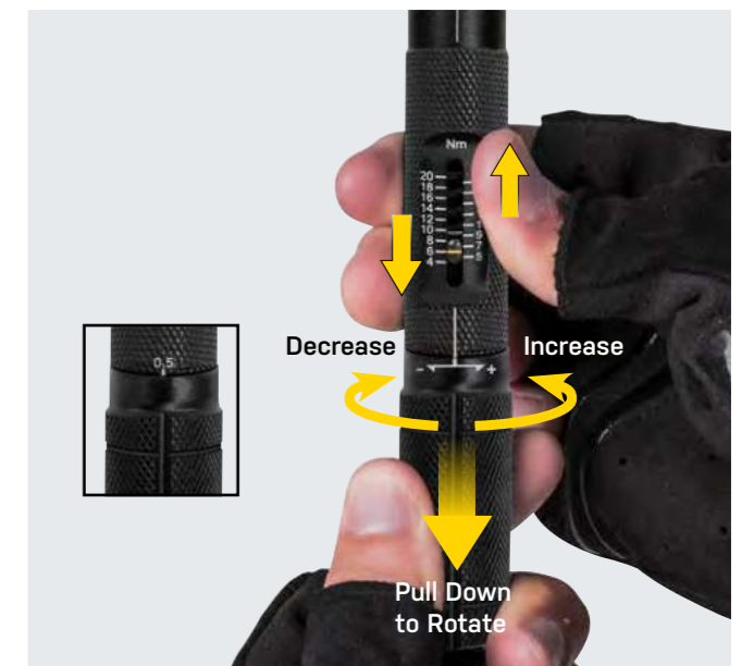
Rotate a half turn for 0.5Nm adjustment
