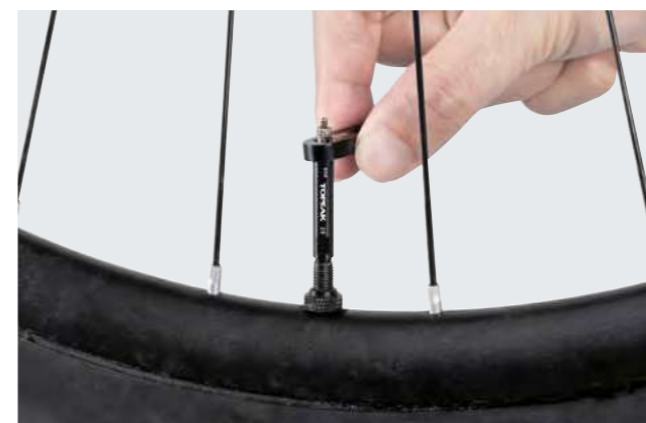
Use Valve Tool to tighten Presta valve core
