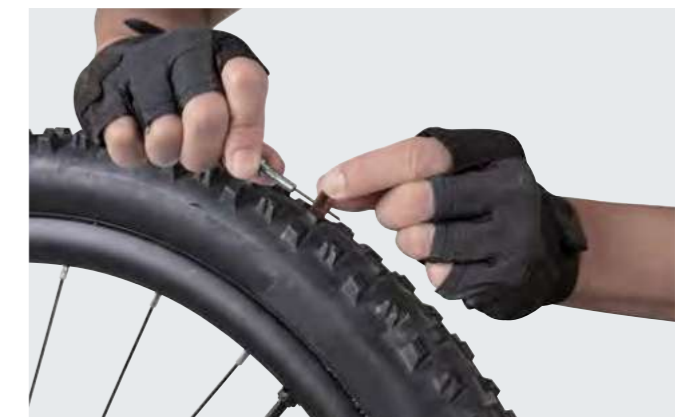
4. Remove excess plug with knife
