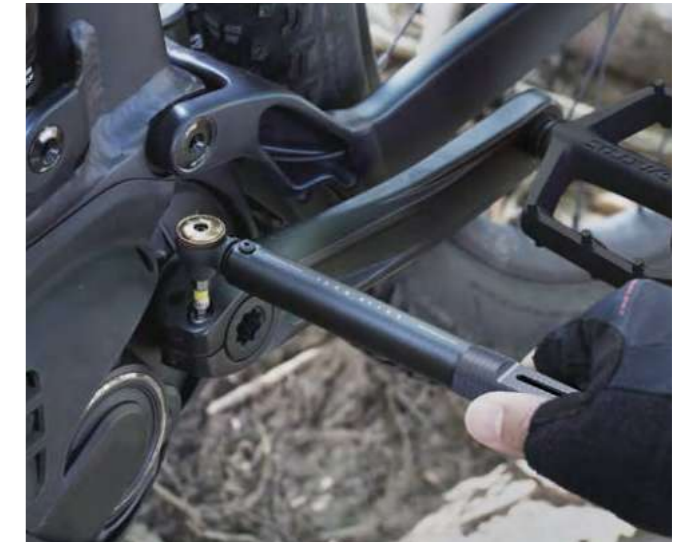
Torque wrench with adjustable preset range of 4 - 20Nm
