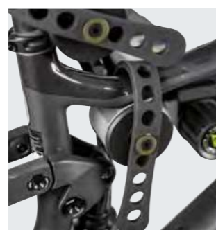
Silicone cups eliminate possible crushing or damage to thin-walled and aero-shaped tubes
