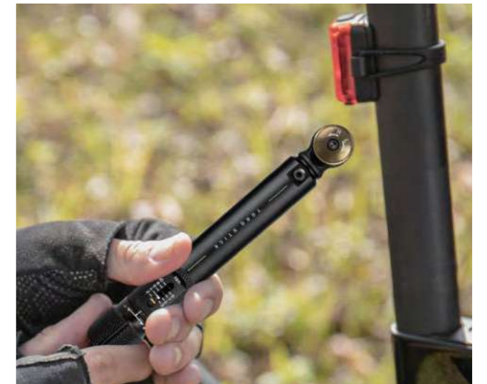
Torque wrench with adjustable preset range of 2 - 10Nm
