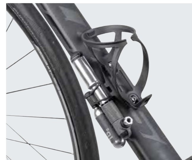
Comes with side mount bracket allowing pump and CO 2 cartridge to be mounted on bike
