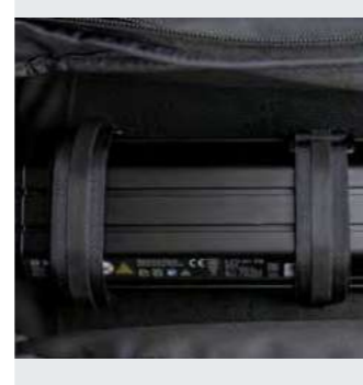
Hook and loop fasteners secure spare battery
